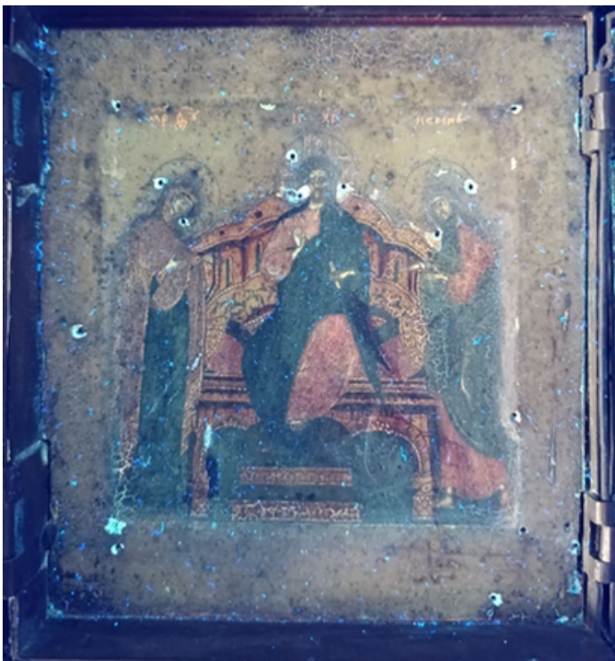
Central panel, UV for the study of superimposed substances
