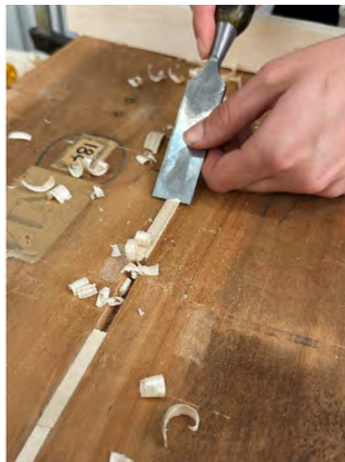
Preparation of the new wedges
