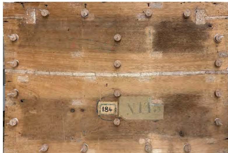
Photo 11 - Bonding the wooden bases with nylon threaded screws
