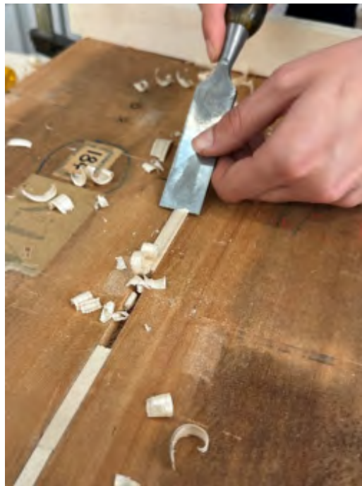
Photo 8 - Machining of the restoration wedges
